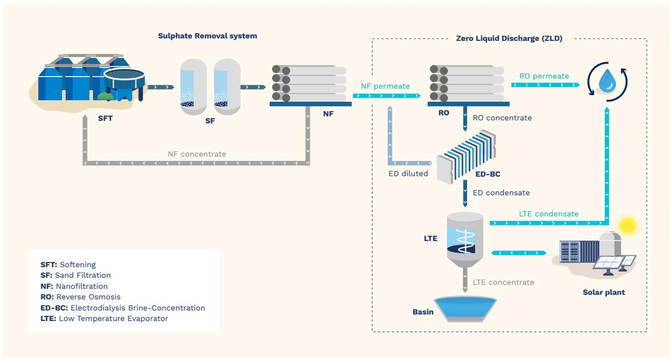
**Figure 4.** Sulphate removal system & ZLD plant scheme.
