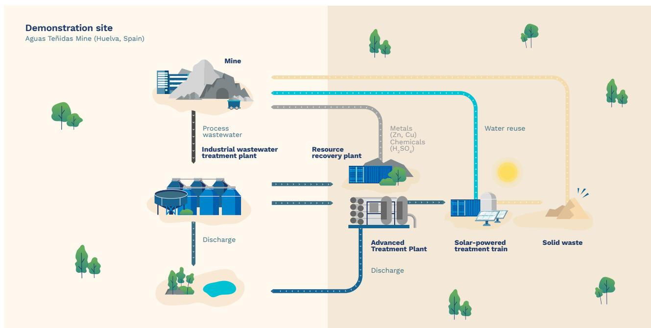
**Figure 1.** Transformation of a linear operation mining scheme into a circular process in REMINE WATER.
