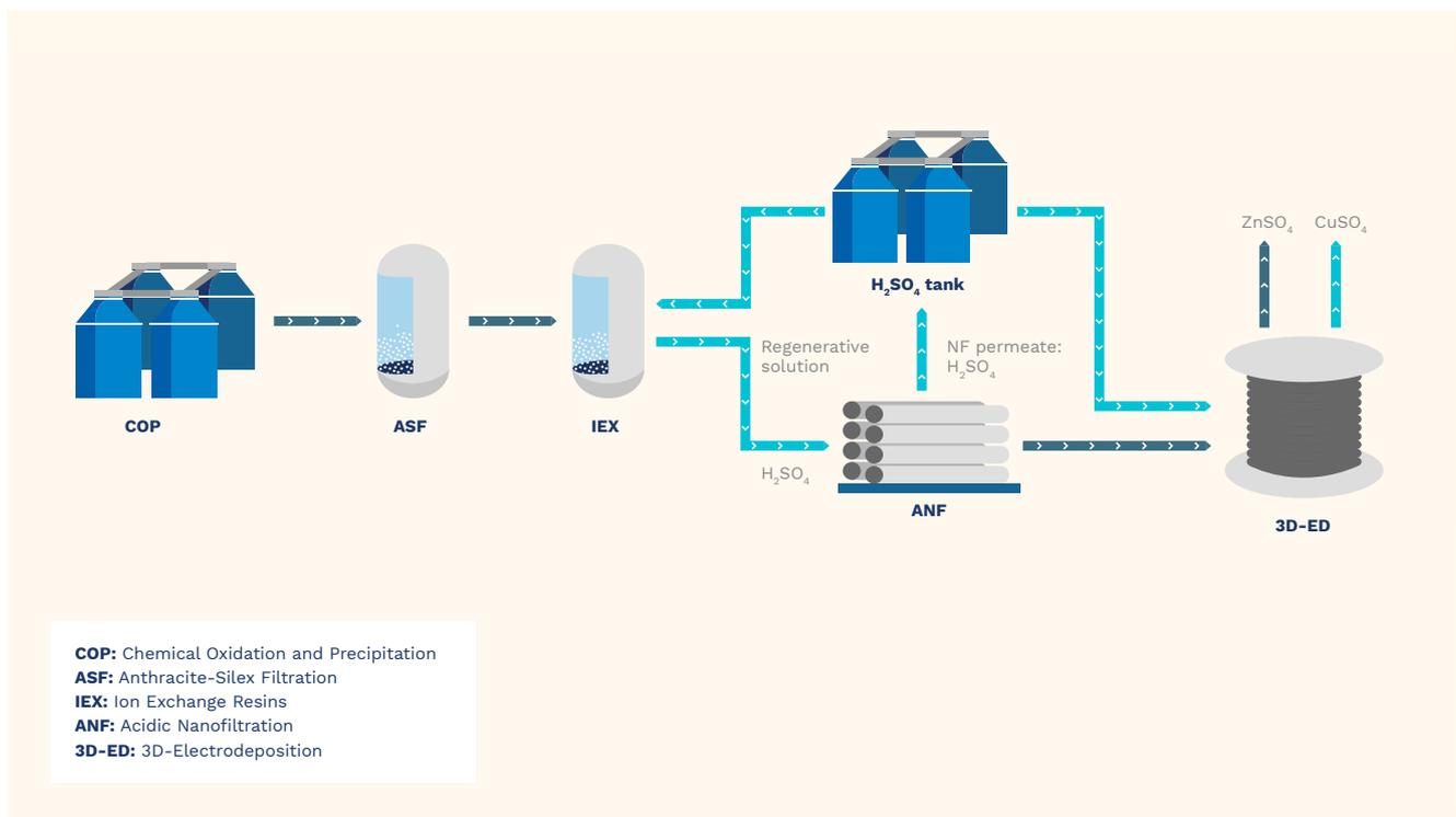
Figure 6. Resource recovery plant scheme.
