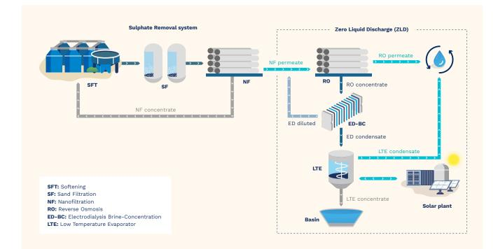
Figure 4. Sulphate removal system & ZLD plant scheme.
